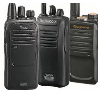
Users of handheld dPMR radios have the choice of using the extra range possible or, if battery life is important, reducing the transmit power to give normal range and get longer battery life.
