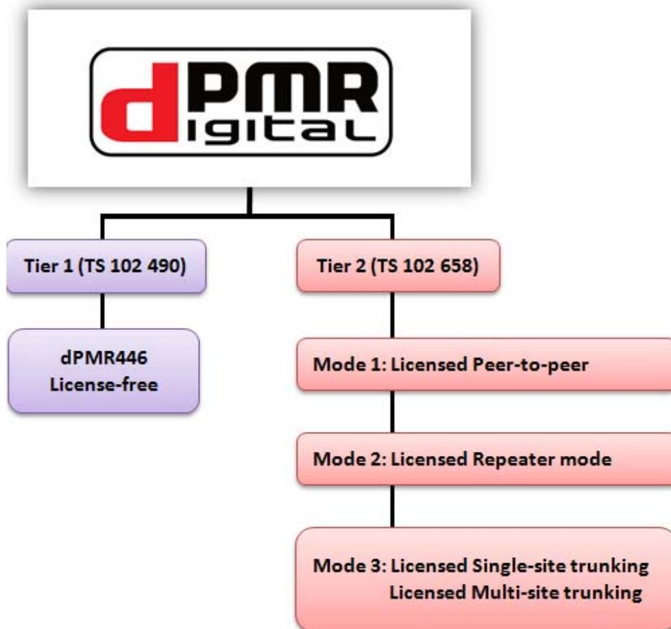
As the diagram shows, dPMR™ is a full featured system capable of providing communications solutions ranging from license-free all the way up to multi-site trunking networks.
