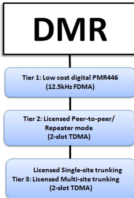
As the diagram shows, DMR is a full featured system capable of providing communications solutions ranging from license-free all the way up to multi-site trunking networks.
