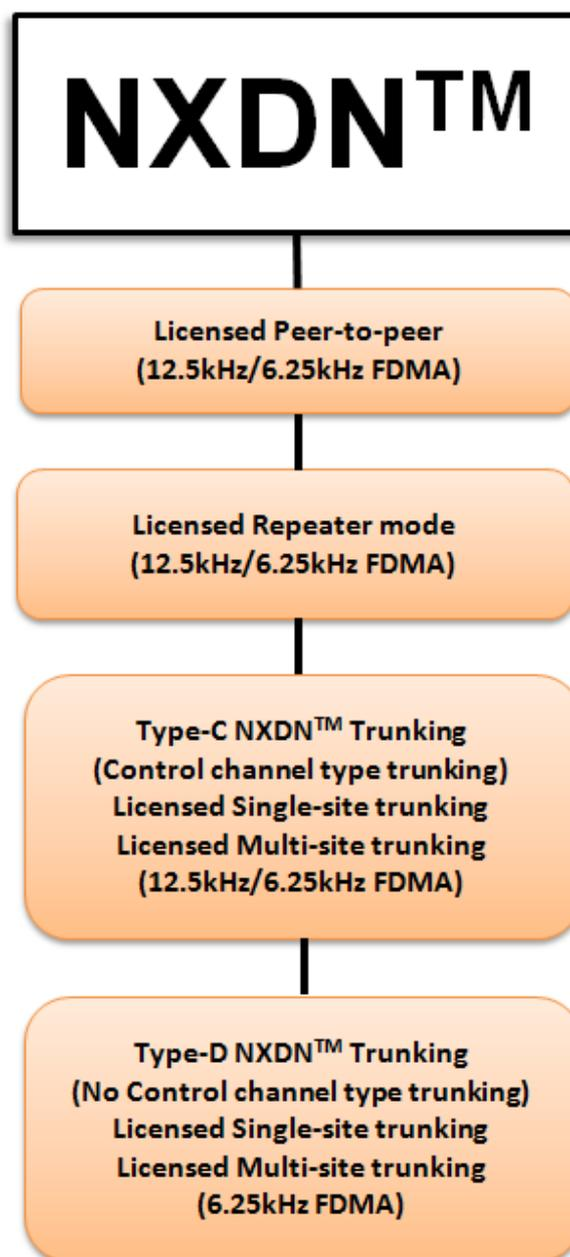
As the diagram shows, NXDN™ is a full featured system capable of providing flexible trunking solutions for small to medium sized networks.
